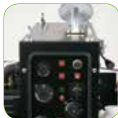
Safety check-up on engine with indication of: - no fuel; - engine shut down due to lack of lubrication/fuel; - inadequate battery charge.
